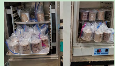
SOIL SAMPLES DRYING IN OVEN
