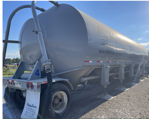
FIGURE 3. PIG PROPERLY STABILIZED WITH ALL SUPPORT LEGS LOWERED
